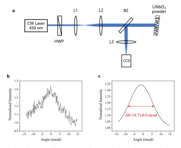
**Fig. S1** (a) Experimental setup used for the measurement of TMFP. HWP, half wavelength plate; L1~3, lens,  $f_{1-3} = 50$ , 200, and 50 mm; BS, beam splitter. (b) The intensity cross-sections of the back-scattering cone recorded by CCD. (c) The Gaussian fit to the data of (b).
