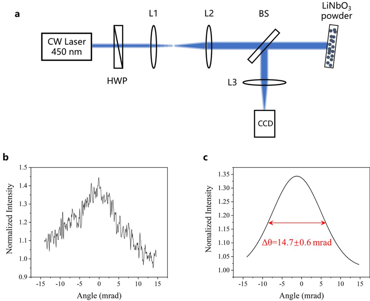
**Fig. S1** (a) Experimental setup used for the measurement of TMFP. HWP, half wavelength plate; L1~3, lens,  $f_{1-3} = 50, 200, \text{ and } 50 \text{ mm}$ ; BS, beam splitter. (b) The intensity cross-sections of the back-scattering cone recorded by CCD. (c) The Gaussian fit to the data of (b).
